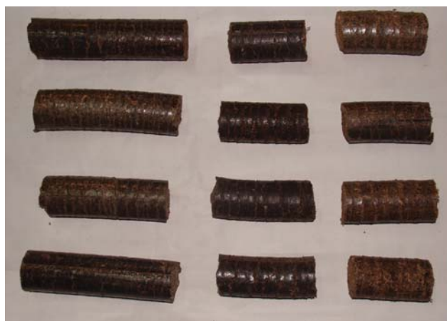
Briquettes made of mustard stalk, mixed waste and wood waste with pressmud
