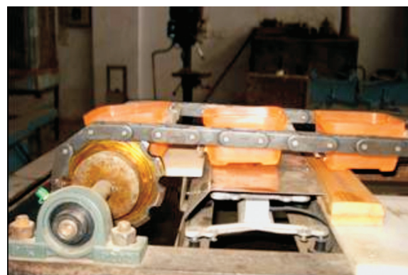
Orange grader under fabrication in the workshop
