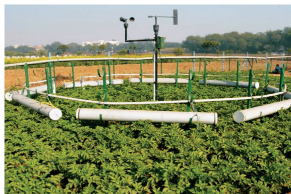
FACE ring with anemometer and \text{CO}_2 supply system
