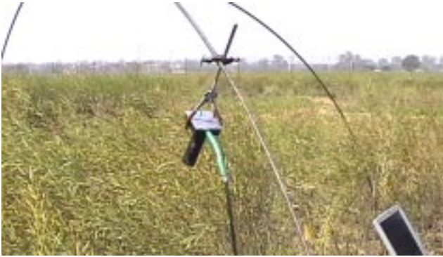
Modified spectroradiometer sensor assembly measuring bidirectional reflectance of mustard crop for further use in retrieval of plant parameters inverting radiative transfer model
