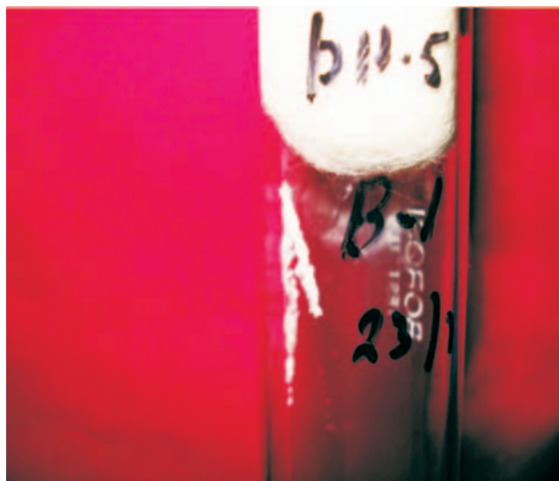
Fibre formation or serration in plastic strips near the top of the tube inoculated with sewage soil inoculums (0.2M phosphate buffer, pH 5.0)
