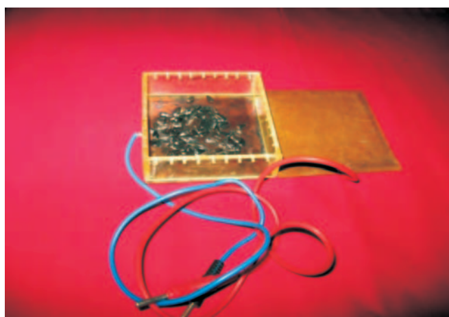
Set up for electric field treatment of sunflower seeds
